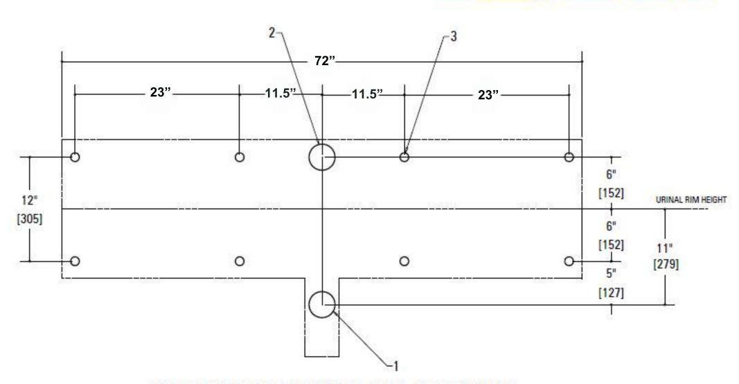
HOLES FOR CORE DRILLING OR STEEL PLATE WALLS
